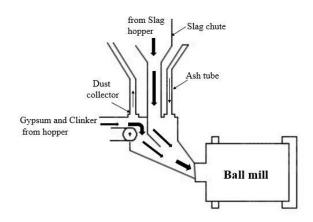
In normal, slag flows in feeder. Separate slag chute method is nothing but a separate chute to slag that flows on feeder and doesn't allow mixing with clinker hot duct. By using this method coating, formation of chute and feeder can be avoided
